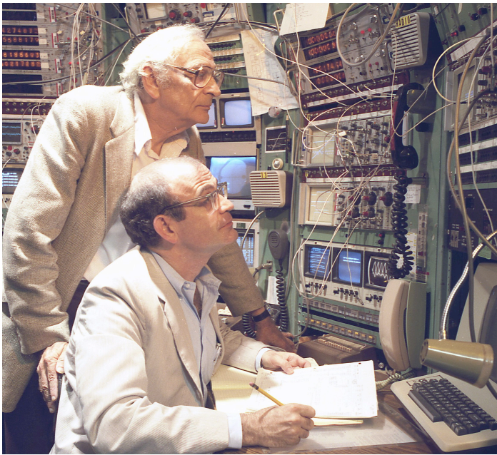
Alan Krusch and Larry Ratner adjusting the timing of betatron tune jump and the strength of the dipole correctors in the AGS MCR.
